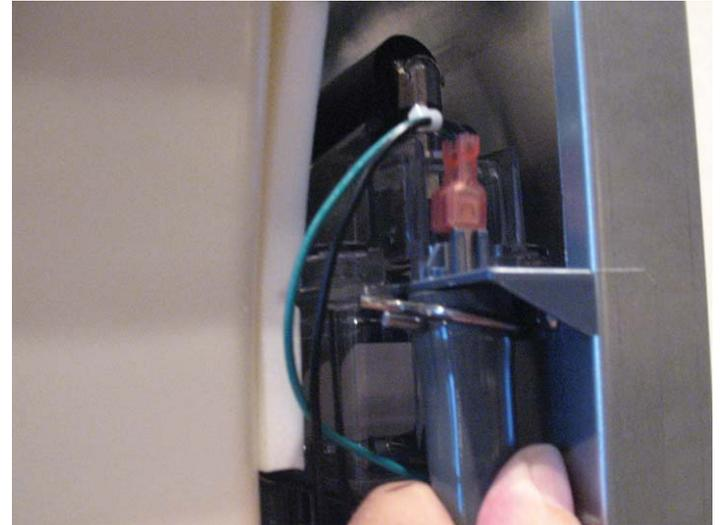
4. Locate drain hose, lower to drain water.
